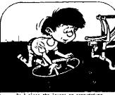
2) I place the levers or screwdriver between the edge of the tire & the me-tallic rim, on which I press to remove the tire.
